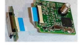
3. Install circuit boards into case being careful to properly seat them in their correct position. Be sure the SMA antenna connector has a black ring installed, then close the case by snapping the case pieces together. Spin the nut on the SMA connector until it touches the case plus ~1/8 turn - do not over-tighten.
