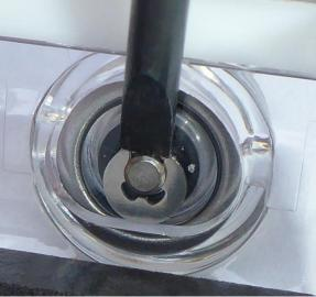
3. Press the button inward to release spring tension and completely remove the C-shaped clip from the shaft, then remove all remaining button pieces from the case.
