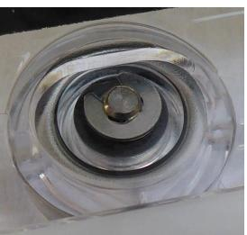
2. Spin the button until the open ends of the C-shaped clip are pointed out of the backdoor. Using a flat screwdriver, push the open ends of the C-shaped clip toward the center shaft. Be cautious not to scratch the plastic with the screwdriver. The surface must remain smooth for proper adhesion of the air vent, otherwise water may pass behind the vent.
